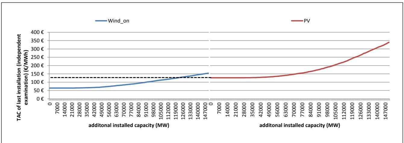
**Fig. 2:** Total average cost (TAC) of directly usable energy in the development of onshore wind power and PV in Germany with independent evaluation of both technologies (feed-in and load profile from 2011; installed wind and PV capacity as of 31.12.2012, Costs based on F-ISE, 2012)
