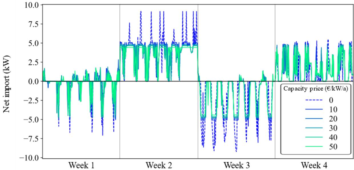
Figure 1. Flexible operation of one building under various capacity price levels.
