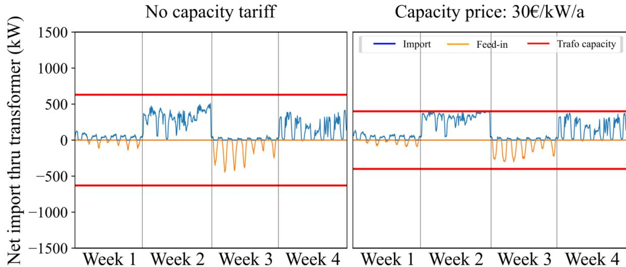
Figure 2. Influence of capacity pricing to the transformer size requirements.
