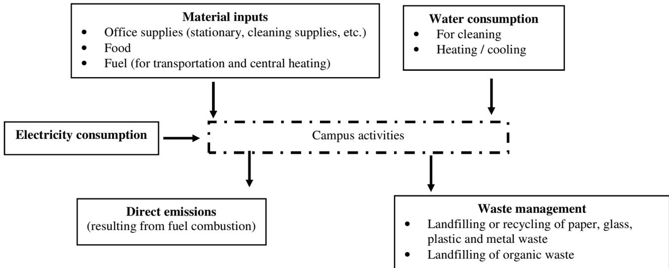
**Figure 1.** System boundaries for the calculation of the carbon footprint of the campus
