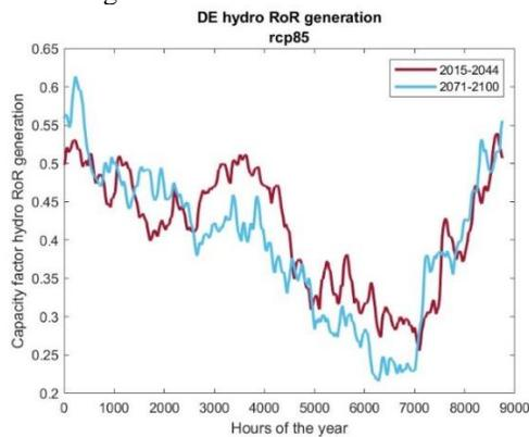
Figure 2: Hourly capacity factor of the hydro RoR generation in Germany in the RCP8.5 scenario for 30 weather years around 2030 (red) and at the end of the century (blue).
