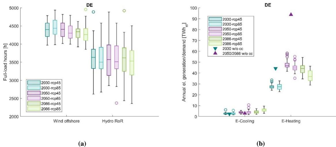
Figure 1: Wind offshore and hydro RoR FLH [h], and e-cooling and e-heating demand [TWh<sub>ei</sub>] for the RCP4.5 and RCP8.5 scenarios and without climate change impact (“w/o cc”). Each boxplot shows the 30 climate years around the displayed year: 2030 (2015-2044), 2050 (2035-2064), and 2085 (2071-2100).
