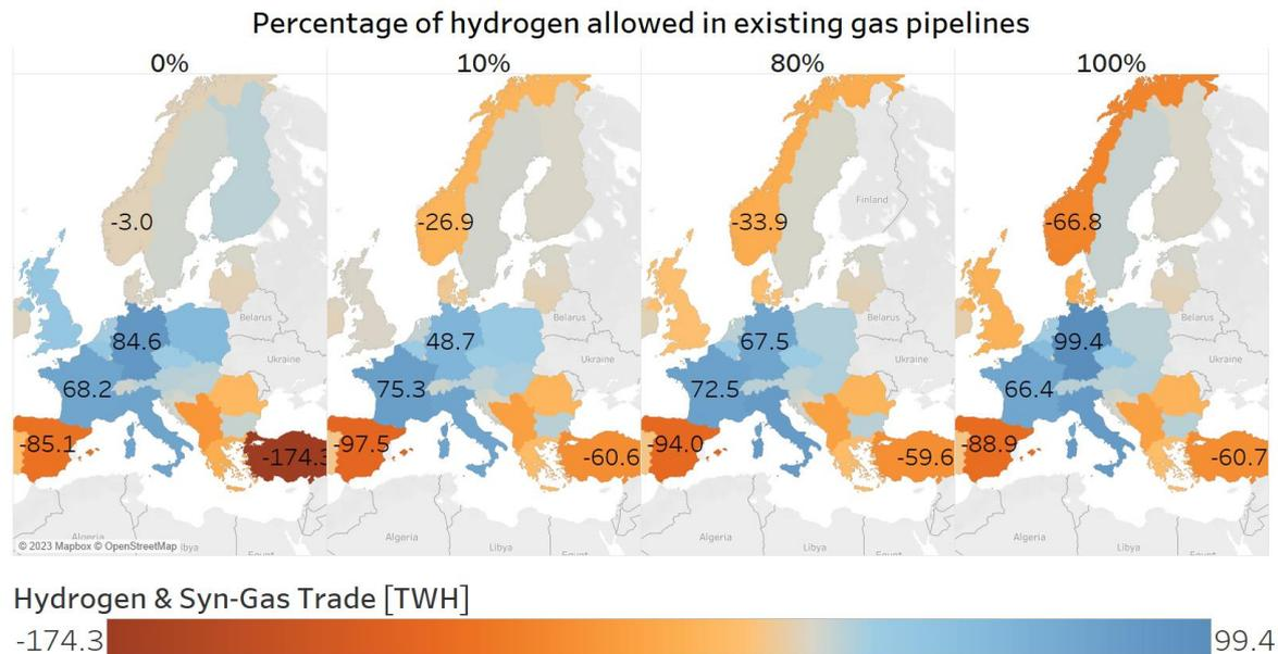
Figure 1: Hydrogen & Syn-Gas Trade at different percentages of hydrogen allowed in pipelines
