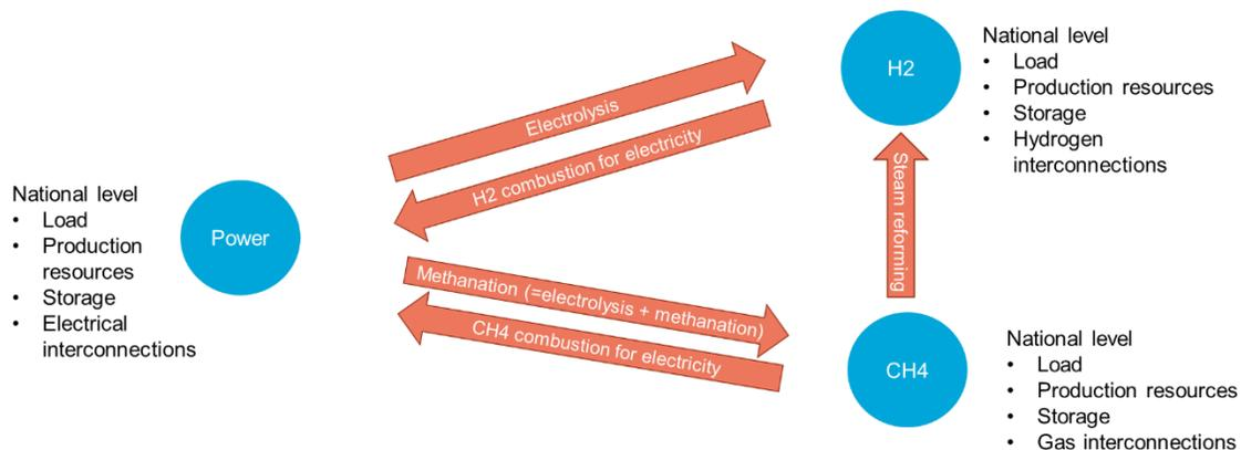
Figure 1 - Simplified representation of the simulated energy system
