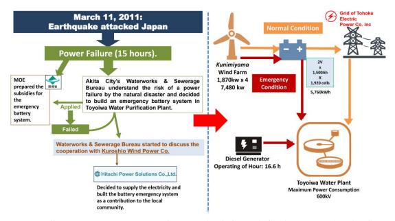
Fig. 2 Emergency power system for water plant before and after the Japan Earthquake of 2011
