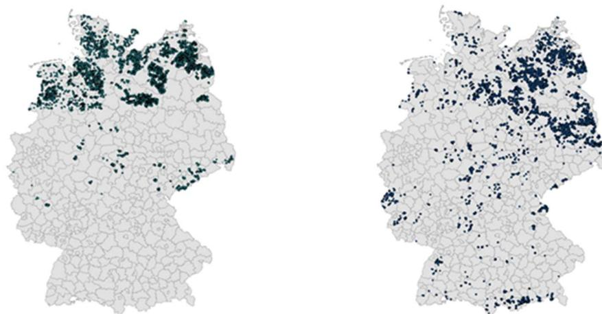
Figure 2: Resulting distribution pattern of onshore wind turbines in Germany for a generation cost minimal allocation (left side) and a residential costs minimal allocation (right side) for a wind generation target of 200TWh/a.
