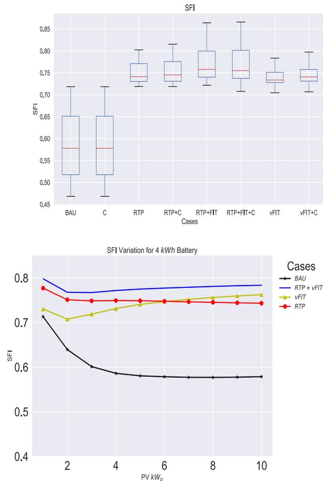
**Figure 1: System-friendliness (SFI) of PV battery systems for different regulatory regimes**
