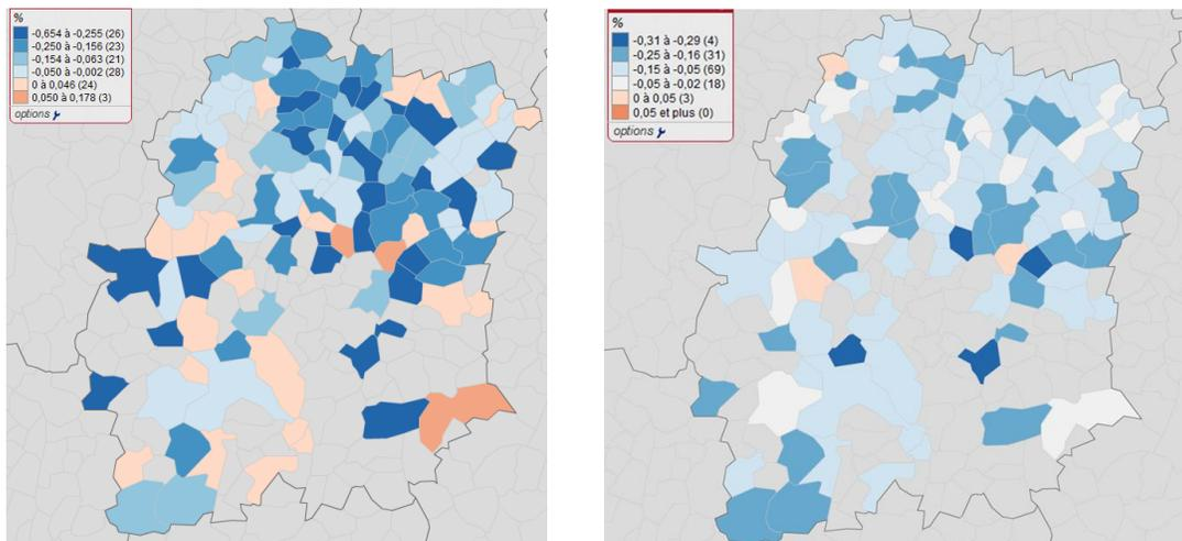
**Figure 2 : Electricity demand forecasting at the municipality level, up to 2035 for a French department (Essonne). On the left: With 90 manufacturing sub-sectors | On the right: With only 6 large manufacturing sectors. (Grey area represents municipality without manufacturing sector)**
