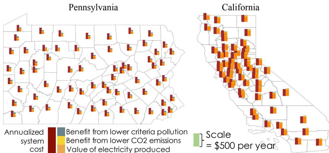
**Figure 1: The figure shows the benefits and costs associated with installing 1kW of PV at different locations in PA and in CA. Left bars represent costs and right bars benefits. Costs are the system installation costs. Benefits include value of electricity generated and reduced pollutant emissions.**
