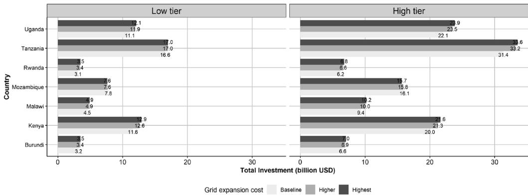
Figure 13: Grid infrastructure expansion costs sensitivity analysis on total capacity.
