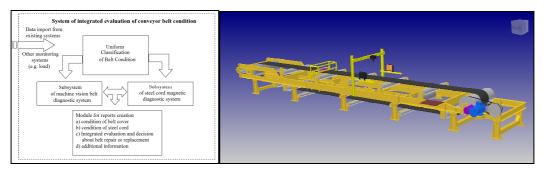
**Fig. 2:** Left: Integrated belt condition diagnostic system utilising information from magnetic and machine vision subsystems. Right: Special testing belt conveyor (Blazej & Jurdziak 2011)
