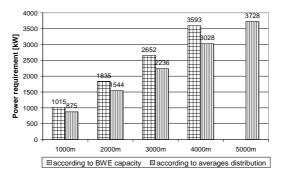
Fig. 3: The differences of required drive power between the standard driving force calculation (full bucketwheel-excavator capacity) versus 97.5% quantile of averaged maximums (computed upon the recorded distribution of actual volume capacity of the BWE) (Gladysiewicz & Kawalec 2006)
