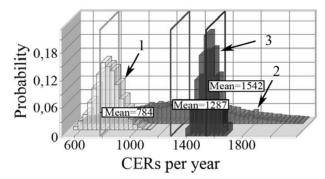
Fig. 1. The Volume of CERs per year (Installed Capacity 500 kW). 1. Solar Generation 2. Wind Generation 3. Hydro Generation
