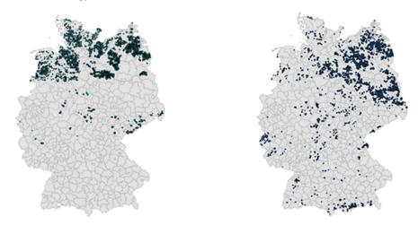
Figure 2: Resulting distribution pattern of onshore wind turbines in Germany for a generation cost minimal allocation (left side) and a residential costs minimal allocation (right side) for a wind generation target of 200TWh/a.
