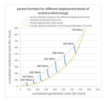
Figure 1: Cost curves and pareto frontiers of an allocation of onshore wind turbines in Germany for different deployment levels of wind energy in TWh.
