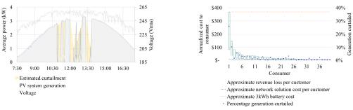
Fig. 1 – Estimated PV curtailment
