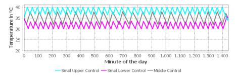
Figure 1: Temperature of the hot water tank for the three control strategies
