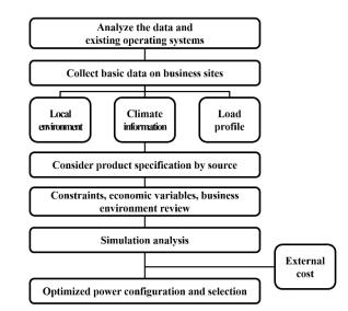
Figure 1. Energy-isolated island generation mix framework
