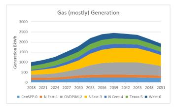
Figure 1. Stacked graph of gas generation by US region due to NGCC replacement for coal.
