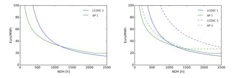
Figure 2: Levelized Cost of Storage Capacity (LCOSC) compared to the Arbitrage Potential (AP) in the Belgian 2015 Day Ahead Market. Storage technology parameters for technology 1 are as presented in Table 1 above. Technology 2 has the same fixed opex, economic lifetime and discount rate, but a capital cost of 600 (kW, a round-trip efficiency of 64% and an energy-to-power ratio of 10.000.
