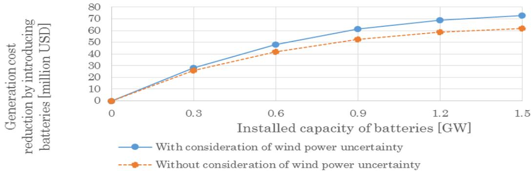
**Fig. 1.** Generation costs reduction by introducing batteries.
