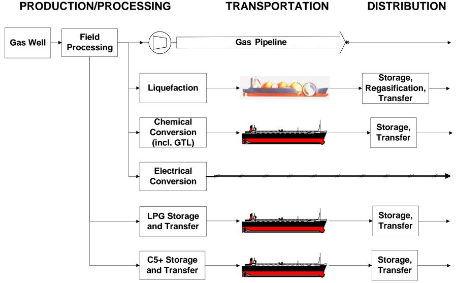
After "Natural Gas Production, Processing, Transport" by Rojey et al.
