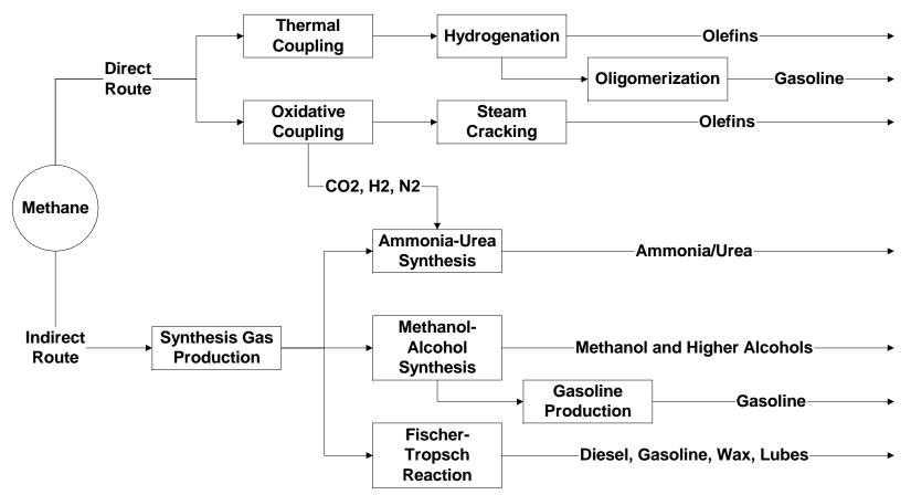
After "Natural Gas Production, Processing, Transport" by Rojey et al.
