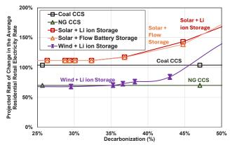
Figure 4. Projected rate of change in the residential retail electricity rate based on the SCoRE model results for each LCA between 25% to 50% CO, emissions abated
