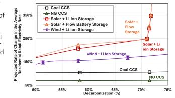
Figure 5. Projected rate of change in the residential retail electricity rate based on the SCoRE model results for each LCA between 50% to 75% CO<sub>2</sub> emissions abated
