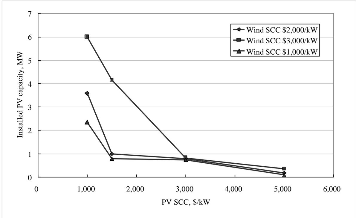
Fig. 8 Capital costs of PV and its installed capacity
