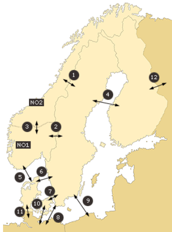
Figure 9: Different zones of Norpool to which market splitting is applied. Connection 1 between Northern Norway NO2 and Sweden represents the two-node model and is frequently constrained.
