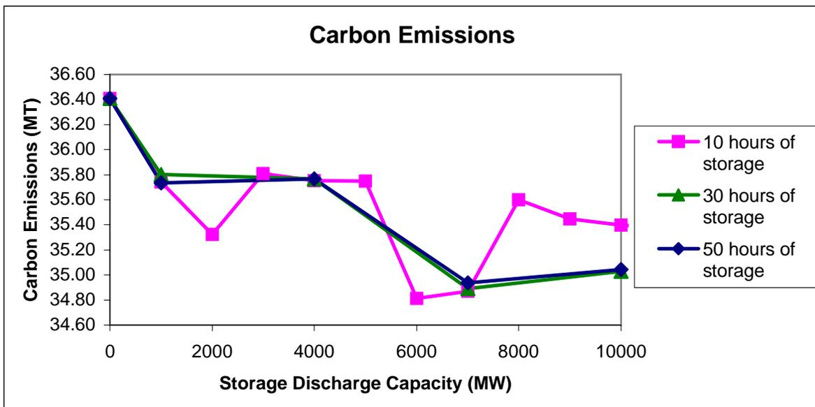
Figure 17. System carbon emissions with various storage capacities.
