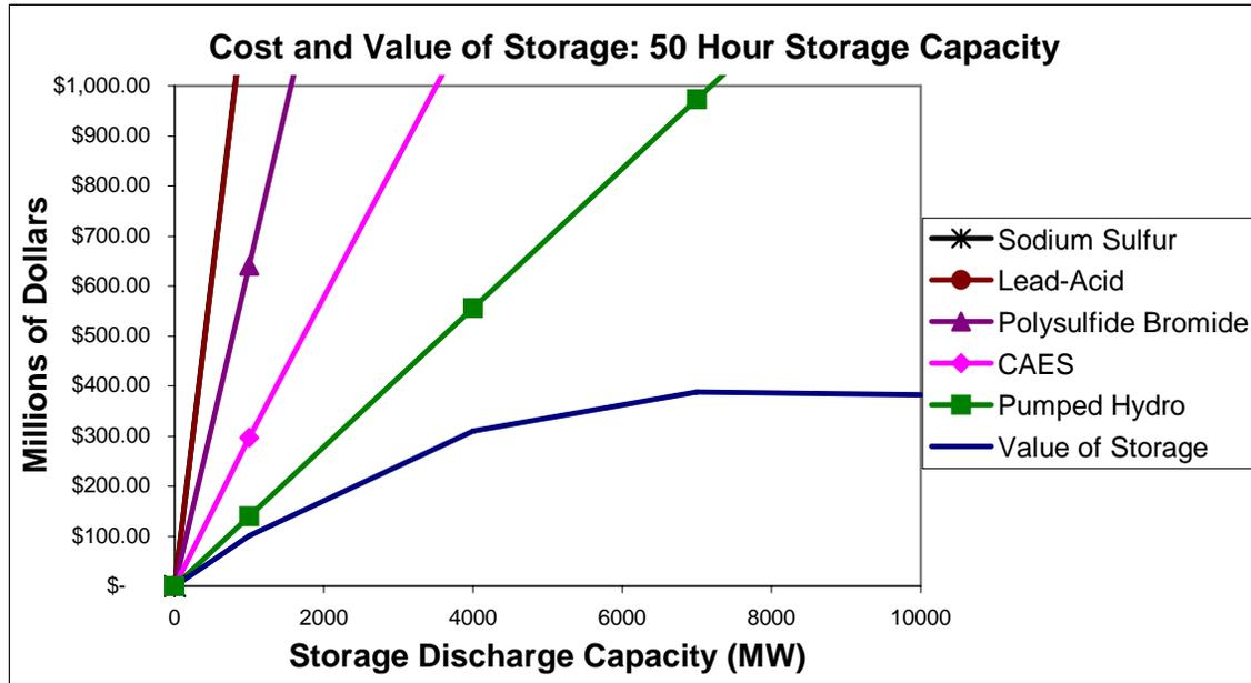
Figure 10. Annual value of technology-neutral storage, with 50 hours of discharge capacity, compared to current costs of actual storage technologies.
