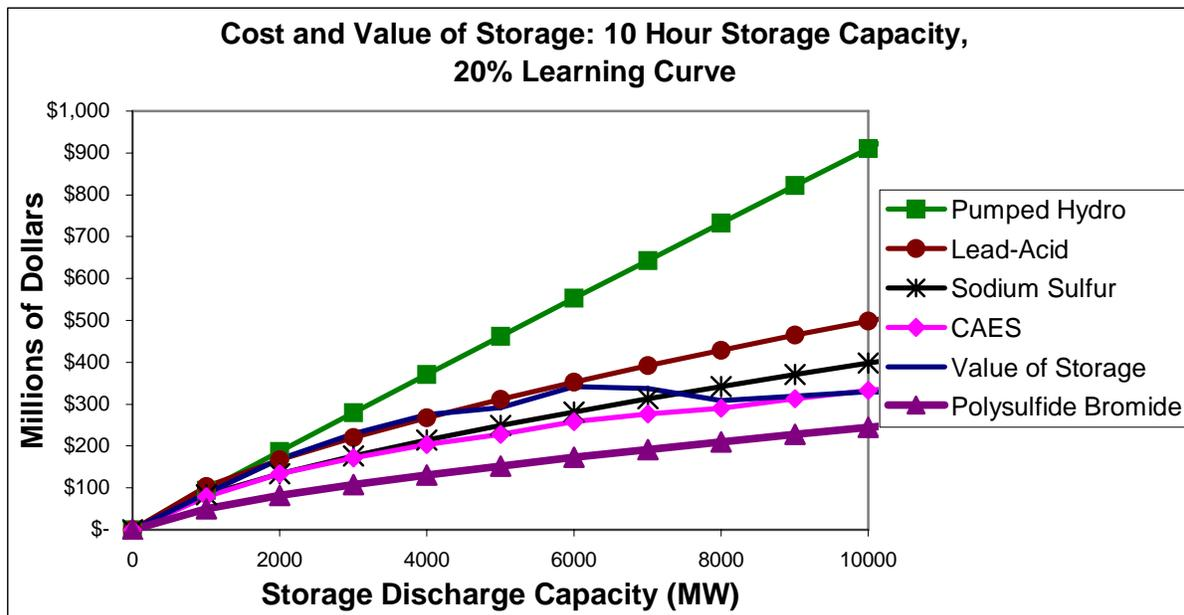
Figure 11. Annual value of technology-neutral storage, with 10 hours of discharge capacity, compared to future costs of actual storage technologies assuming cost decreases according to a 20% learning curve.
