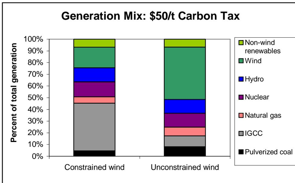
Figure 5. 2020 generation mix with no storage and \$50/t carbon tax. In all model runs but the one presented on the right of this figure, new wind capacity was constrained by high-speed wind resource availability in the state, much of which exists at the four wind sites considered in the model. This constraint limits new wind capacity to about 12 GW, and limits wind penetration to 18%. When the constraint was ignored, new wind capacity increased to 31 GW and wind penetration increased to 45%.
