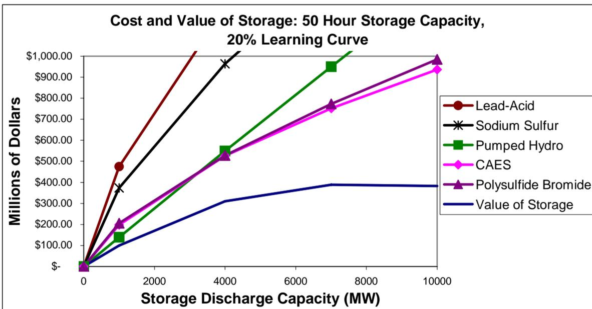
Figure 13. Annual value of technology-neutral storage, with 50 hours of discharge capacity, compared to future costs of actual storage technologies assuming cost decreases according to a 20% learning curve.
