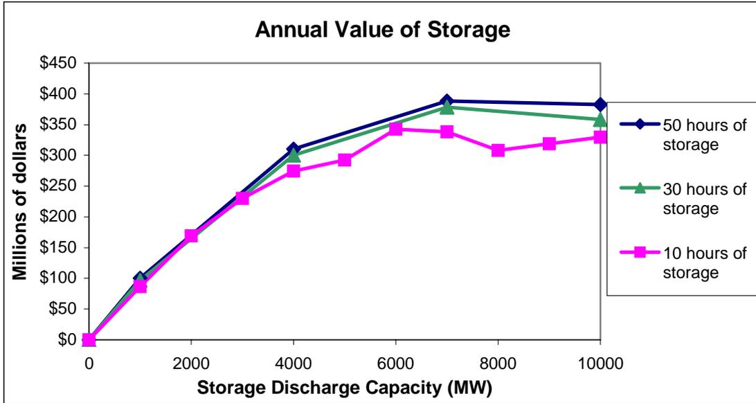
Figure 7. Value of storage. The value of particular storage capacity is the difference between the total system cost with no storage and the total system cost with that storage capacity.
