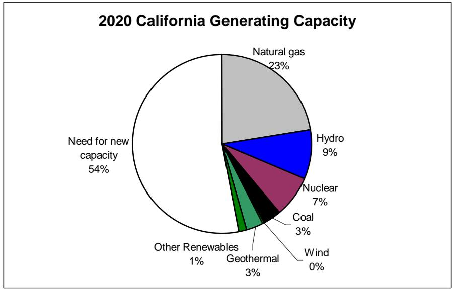
Figure 2. Projected in-state generating capacity mix in 2020. Based on 2004 capacity mix, and assuming retirements according to Table 1. This figure does not take into account demand growth between 2004 and 2020, which will increase the need for new capacity.
