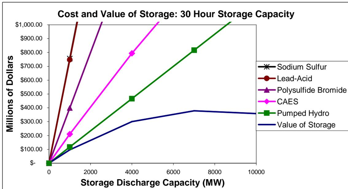
Figure 9. Annual value of technology-neutral storage, with 30 hours of discharge capacity, compared to current costs of actual storage technologies.
