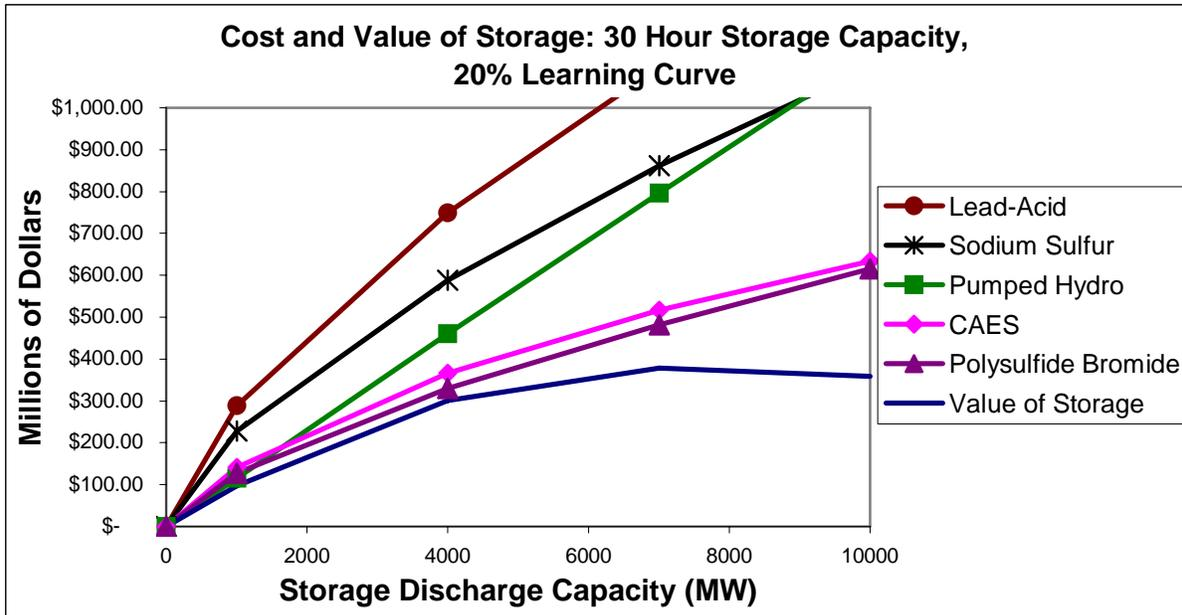
Figure 12. Annual value of technology-neutral storage, with 30 hours of discharge capacity, compared to future costs of actual storage technologies assuming cost decreases according to a 20% learning curve.
