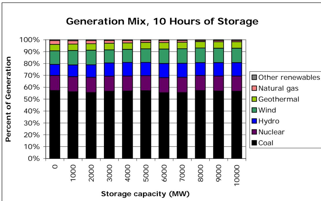
Figure 14. Generation mix with 10 hours of storage and varying storage discharge capacities.
