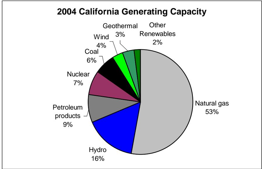
Figure 1. California in-state generating capacity mix in 2004. From CEC 2005b. 81% of California’s electricity demand is met with in-state generation; the rest is met with imports from the Northwest (mostly hydro) and Southwest (mostly coal).
