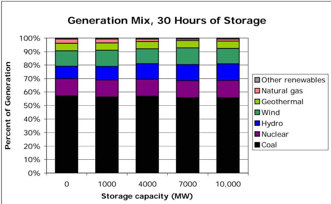
Figure 15. Generation mix with 30 hours of storage and varying storage discharge capacities.
