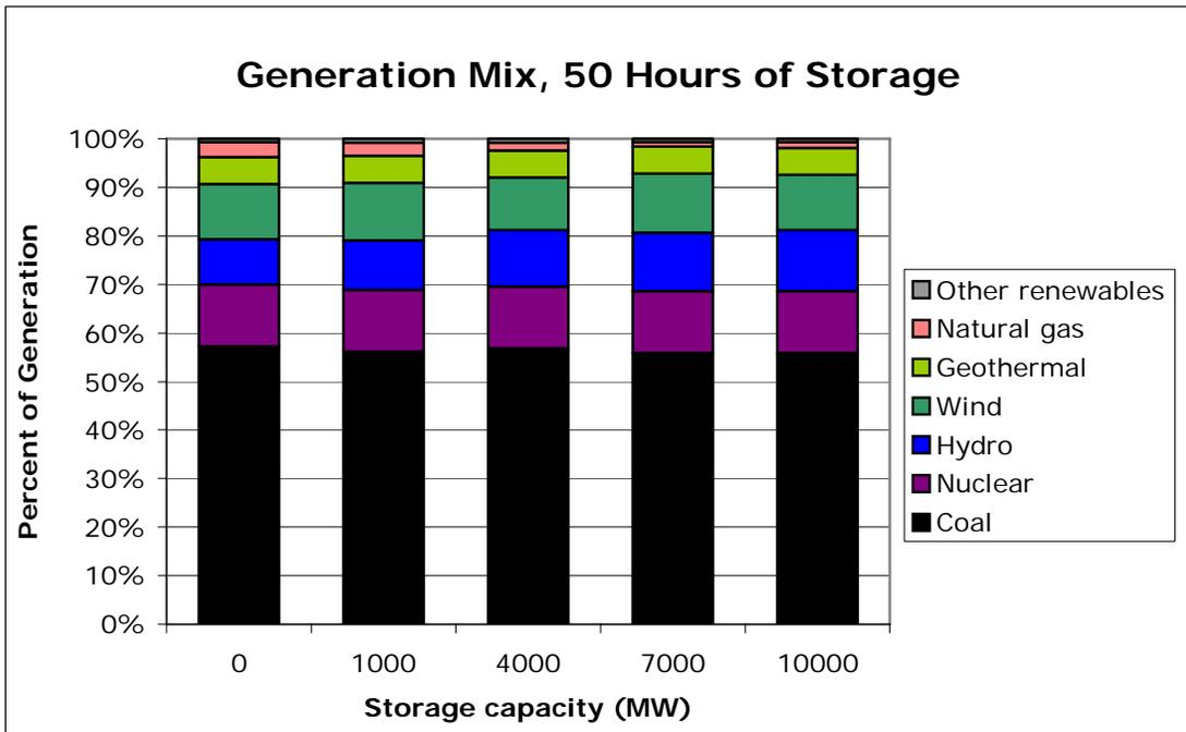
Figure 16. Generation mix with 50 hours of storage and varying storage discharge capacities.
