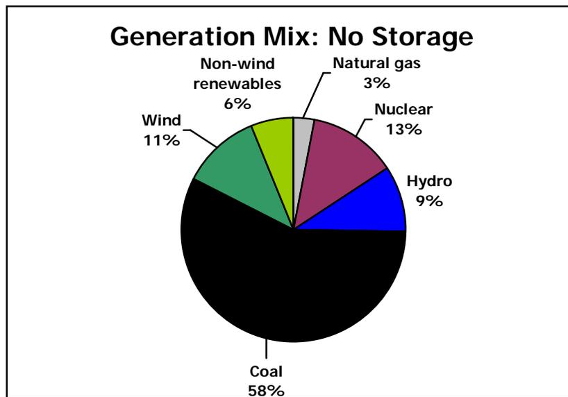
Figure 3. California generation mix in 2020, based on optimal capacities of new generators (see Table 7) and existing generators that have not retired by 2020.
