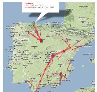
In this figure the emission sources are the green points and the blue points are all the available sinks. The red lines are the routes that link emission sources with sinks. The thickness of each line is proportional to the  $CO^2$  volume transported from the pipeline.
