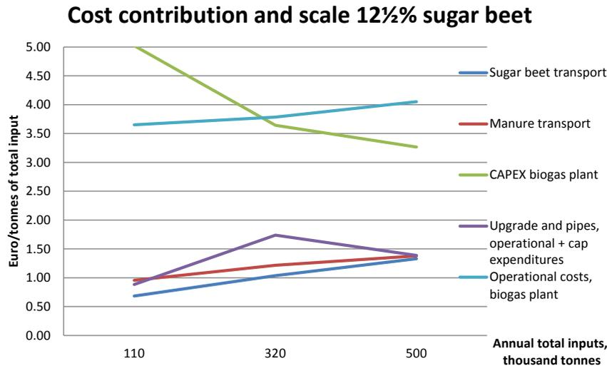
**Figure 1 Trade off between rising operational costs (including transport) and reduced capital costs in a case of mixed manure and sugar beet input and three different scales of operation**
