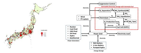
Fig.1 Power grid and demand in optimal power generation mix (OPGM) model
