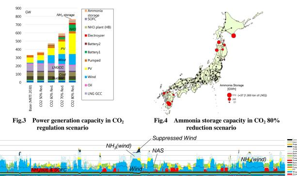
Fig.5 Optimal power dispatch in May at Hokkaido (northern region) under CO<sub>2</sub> 80% reduction scenario
