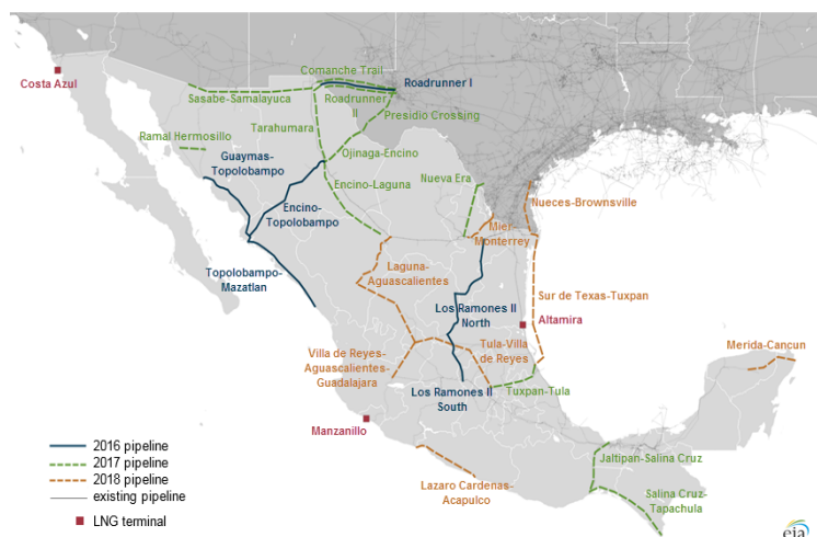
Figure 3. Existing and Proposed Natural Gas Pipelines and LNG facilities in Mexico
