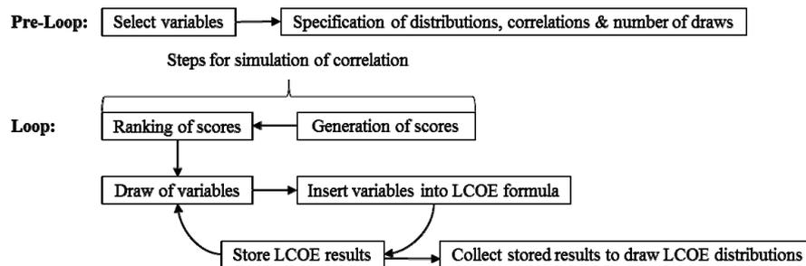
Figure 1: Simulation procedure.
