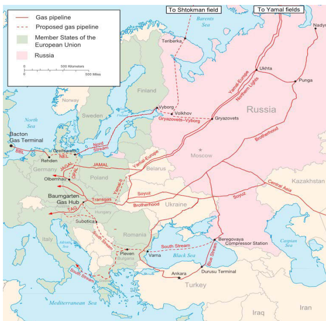
Figure 1. Transit routes for natural gas.
