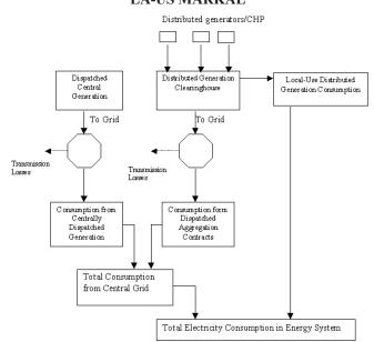
tion (Figure 1). For centrally dispatched generation, over 90 generation technologies are characterized. The generation types characterized include fossil (i.e., oil, natural gas, and coal) steam, combined cycle, and conventional and advanced turbines. As part of this technology choice set, nine 'clean coal' technologies including integrated coal gasification combined cycle, atmospheric and pressurized fluidized bed, and advanced turbines are depicted. Renewable technologies
