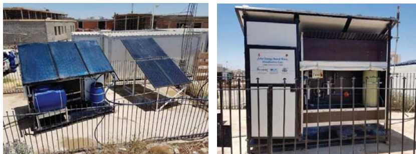
Fig 1. the "MD ORYX" autonomous desalination solar-driven membrane distillation
