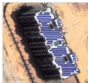
Fig. 2 The designed roof-top PV system
